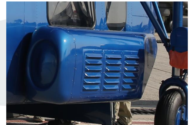
Air conditioning unit
